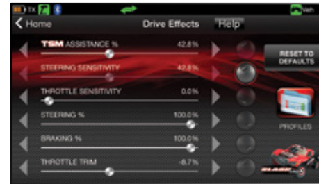
Tap and slide to adjust TSM, Steering Sensitivity, Throttle Trim, Braking Percent, and more!
