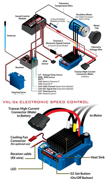
\*\* Accessory sensor expansion port for use with the Telemetry Expander Module (see Traxxas.com and included materials for more information)
