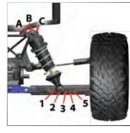
The suspension of your model has been set up for off-road performance (position 2 on the front suspension arms and position 3 on the rear suspension arms). If you plan on driving on hard surfaces the following changes should be made:
