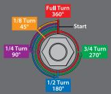
Do not run your model with the slipper clutch adjusting spring fully compressed. The minimum recommended slipper clutch setting is 1/2 turn counterclockwise from fully compressed.
