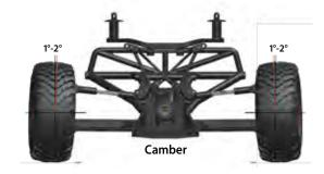
Static Camber Base Factory Settings **Front:** 1° negative camber each side Rear: 1° negative camber each side
